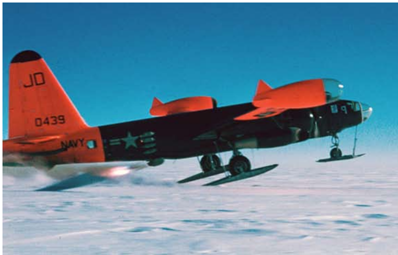
Two turnin', two burnin', sixteen pushin', is how pilots described a Neptune's take-off. The pods at the end of the wings housed radar and navigation gear.
